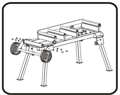
Installation of the Cutter(2) Install the wheels assembly to the base as shown.
