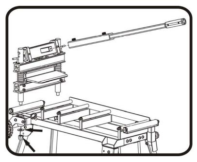
Installation of the Cutter(3) Install the cutter head to the base as shown.
